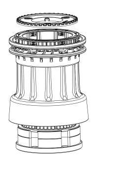
Remove the roller-bearing and the washer. Follow this by unscrewing the five (5) screws locking the centre hub to the base. Depending on the version of the winch, this is done using a hexalobular key size T30 or a 5mm Allen-key.
