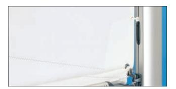
The sail slides are fed in through the spring-loaded gate. When reefing, the sail slides pass through the closed track gate down to the boom, holding the sail in place and facilitating faster and safer reefing. When the spring-loaded section of the track gate is removed, the track gate can just as easily be used with a luff rope.
