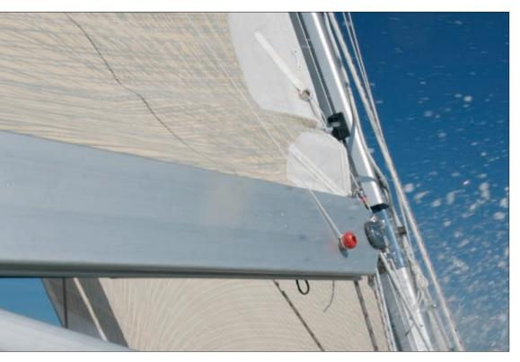
The sail entry gate is designed for use with our MDS cars or with conventional sail slides. When using it with MDS cars, you simply remove the sail entry gate when installing or removing the cars. When using it with conventional slides, use the springloaded mid section of the sail entry gate.
